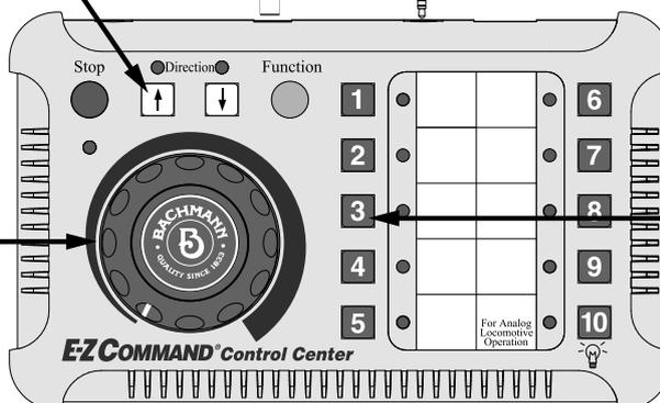
Select decoder address 3 for turntable control or reprogram if desired.
